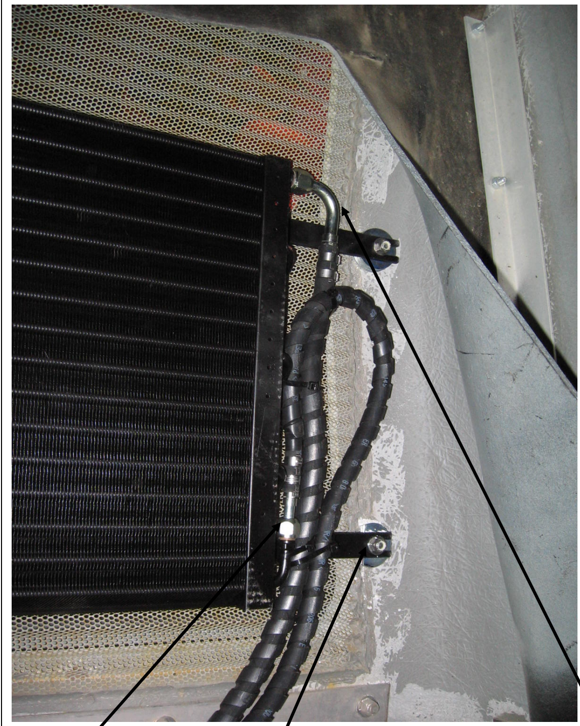
5/16" straight fitting on bottom of condenser.
