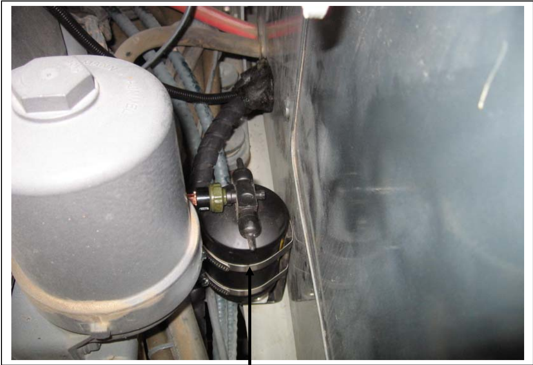
Install drier with binary switch pointing away from the cab.
