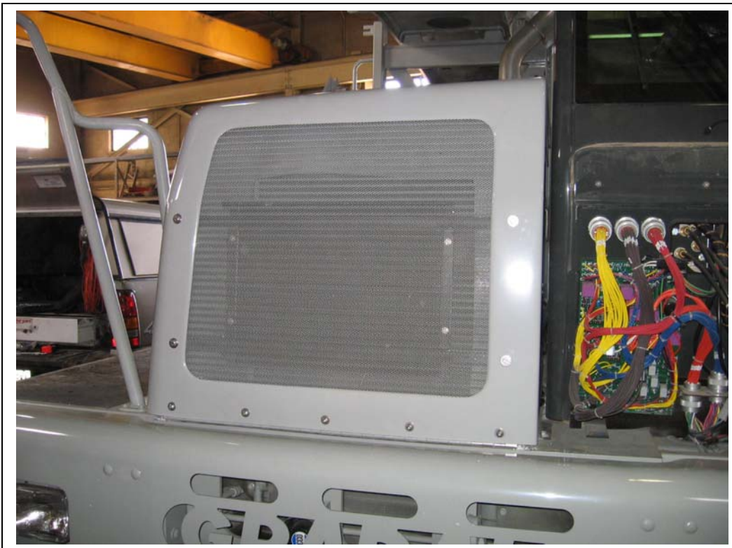
5/16" stainless steel mount bolts on outside of engine hood.
