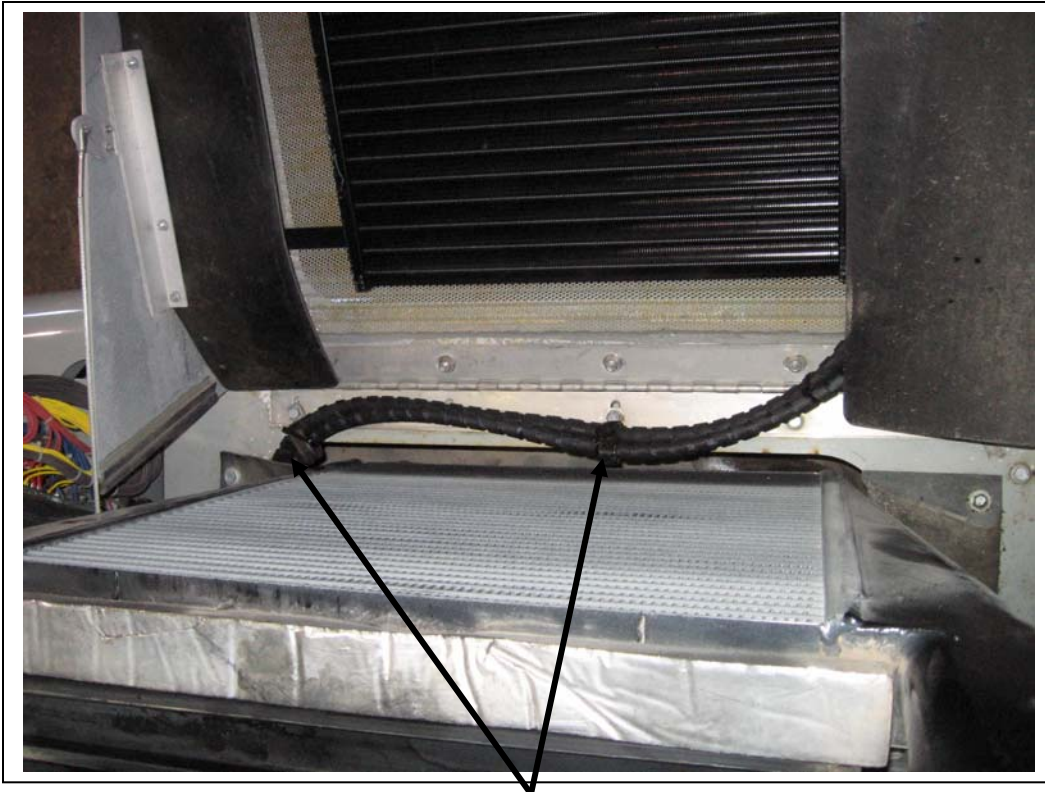
Condenser hose runs through double hose clamps provided in the kit.
