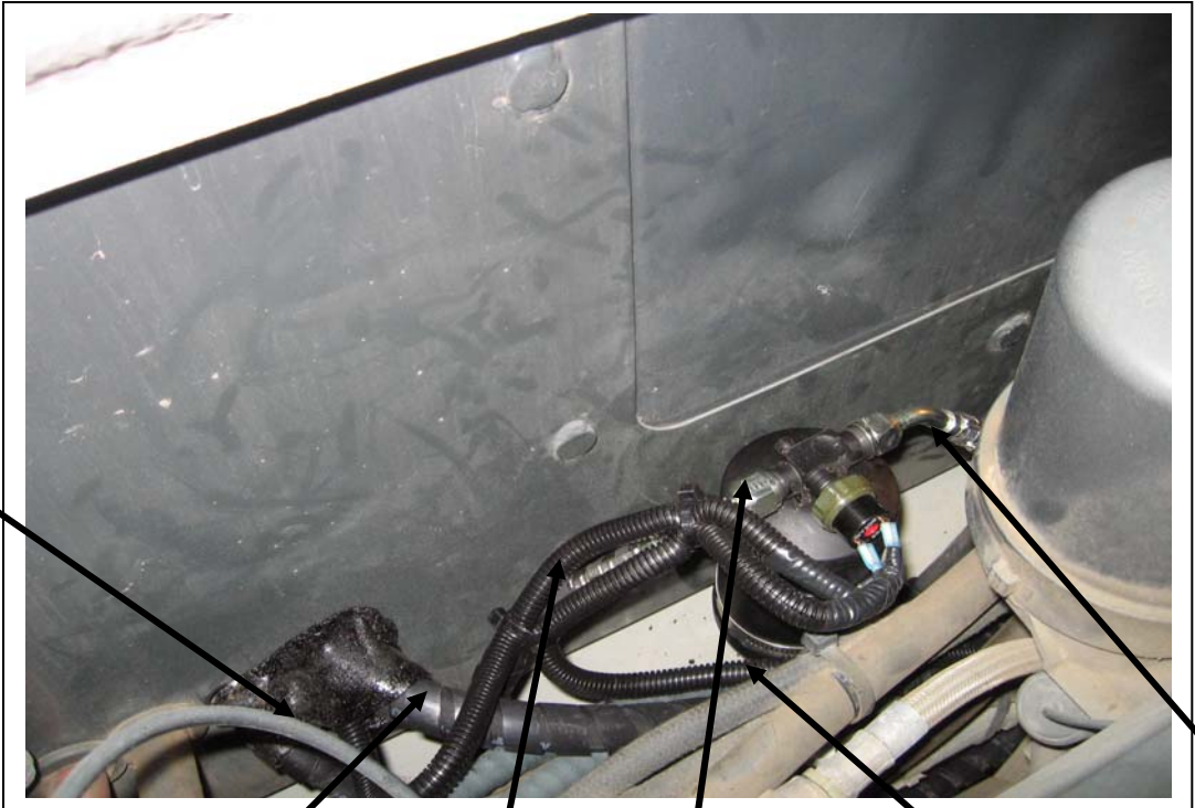
Install drier with binary switch pointing away from the cab.
