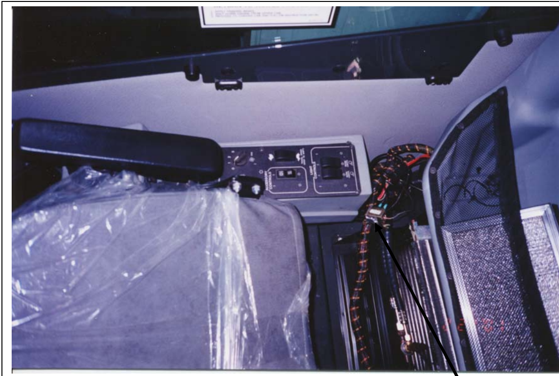
On lower unit installs, an A/C on-off push button switch is installed on the right side of the front dash near the blower switch.
