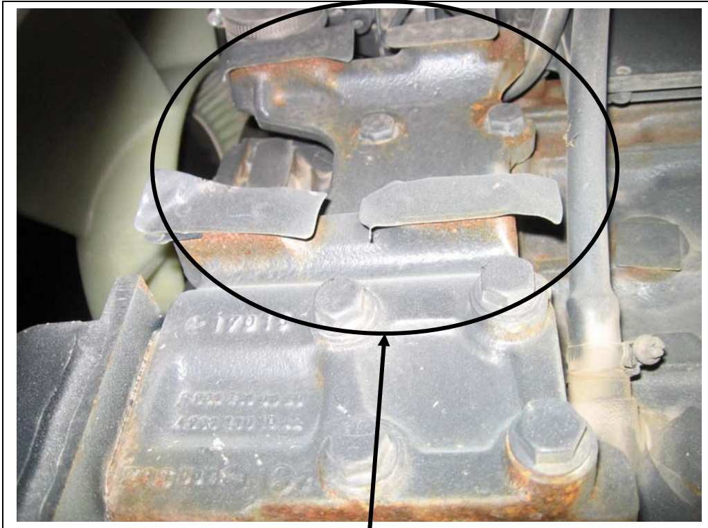
Compressor mount goes here.
