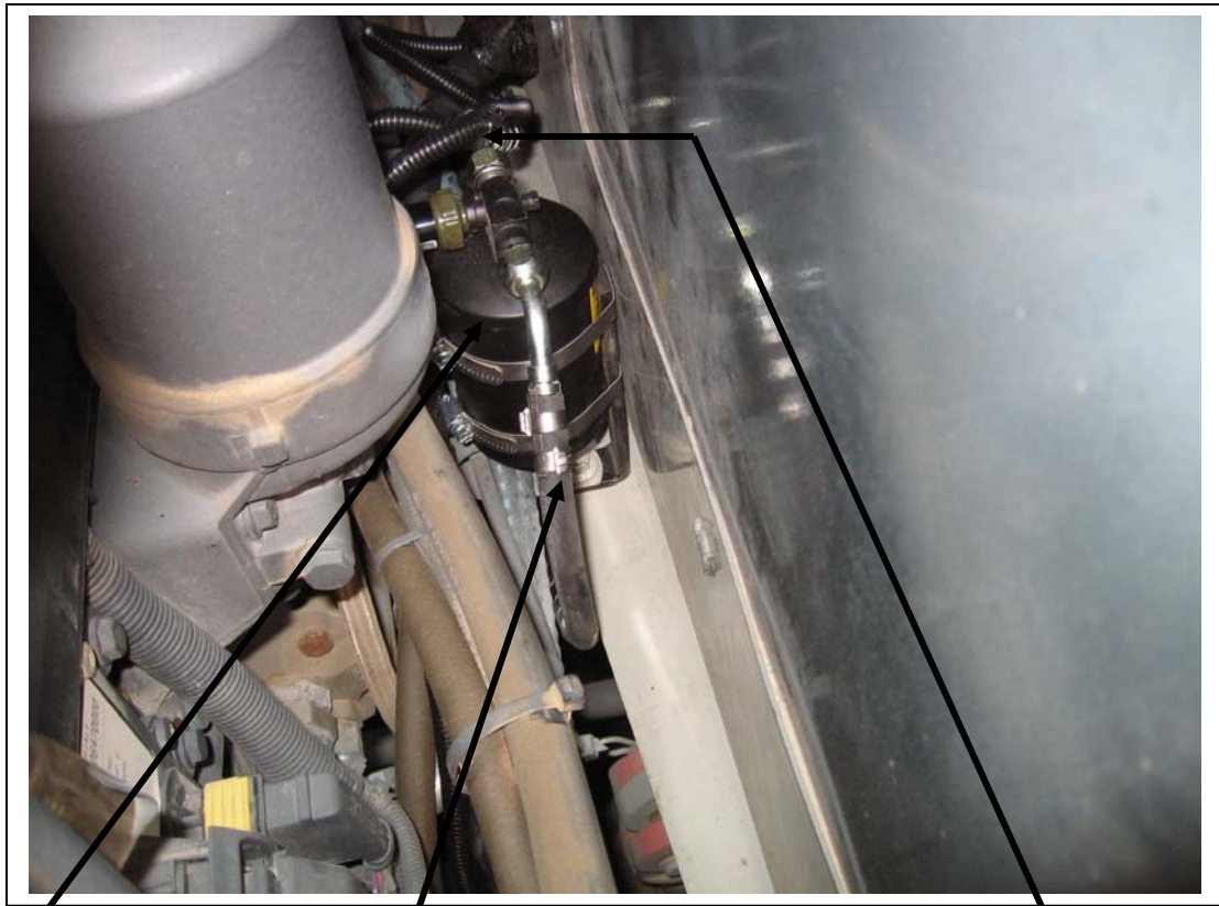
Drier c/w binary switch
